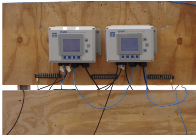
YSI 5500D continuous optical dissolved oxygen monitors mounted for continual DO data. Photo courtesy Texas A&M AgriLife Research Mariculture Lab.
