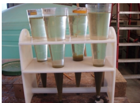
Imhoff cones with bacterial floc used throughout the duration of the study. Photo courtesy Texas A&M AgriLife Research Mariculture Lab.
